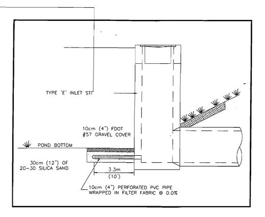
Figure 1. Schematic of dry detention pond outfall structure with anti-clogging device.
